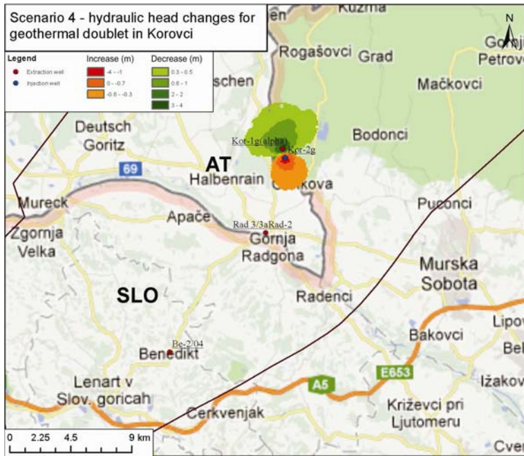
Figure 49. Modelled hydraulic head changes for geothermal doublet in Korovci after 100 years of simulation.
